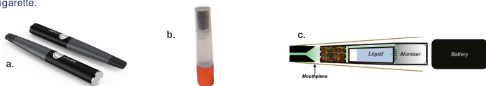
Figure 1. (a) THP device exterior - Features a Li-ion rechargeable battery and single voltage output. (b) THP pod - Disposable cartomiser with e-liquid formulation and tobacco plug. (c) Schematic of THP with hybrid e-cig and tobacco disposable pods - The e-liquid aerosol generated at the coil passes through the tobacco to release tobacco sensory characteristics.
