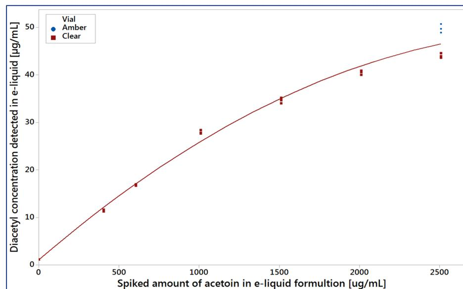
Figure 5: Measured diacetyl concentration in e-liquid 21 days after spiking
