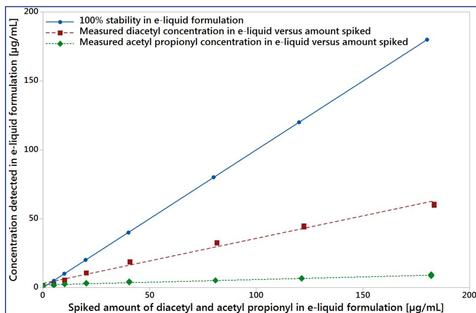
Figure 2. Measured concentration of DA and AP in an e-liquid formulation versus the amount initially spiked into e-liquid
