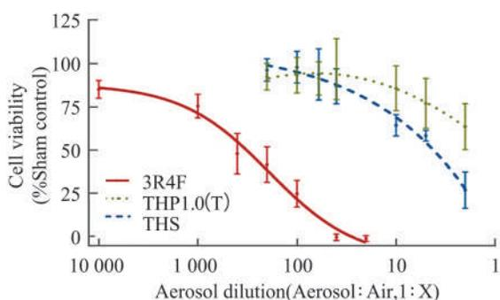
**Fig.4** Neutral red uptake (NRU)-cell viability of H292 lung epithelium after 1 hour exposure to a range of dilutions for the three test products. Error bars are standard deviations for replicates at the same dilution, and the type of curve fitting applied to the data is a non-linear regression.
