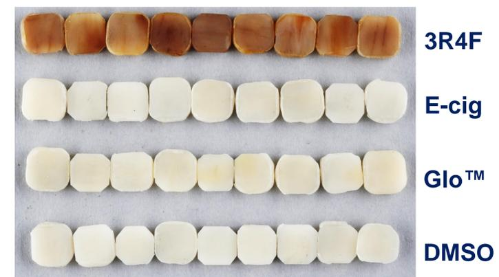
**Figure 4.** Enamel block discolouration after 14 days exposure to TPM generated from 3R4F cigarettes, Glo™ or BAT prototype e-cig and also DMSO control.
