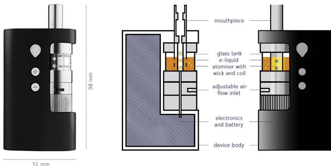
Fig. 1. Pictorial and schematic representation of Vype eBox device (Nicoventures Trading Ltd., UK) size, dimensions and controls.
