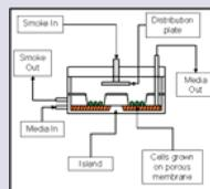
Fig. 3: Schematic Of Exposure Chamber
