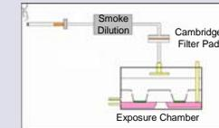
Fig. 8: Removal of particulate matter from whole smoke
