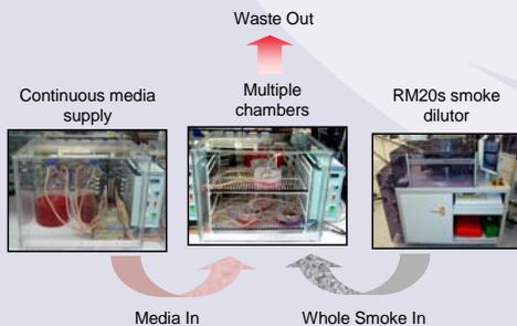
Fig. 2 : Whole Smoke Exposure System
