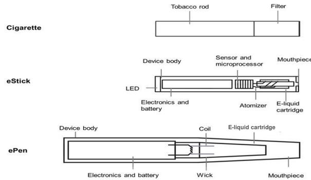
Figure 2: A schematic representation of the three aerosol products used in the study
