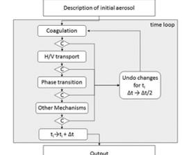
Figure 5 : Key physical processes and their incorporation into Lagrangian / Eulerian dynamic transport model (Pichelstorfer *et al*, 2013)
