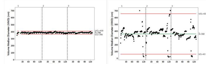
Figure 4 : Droplet diameter precision by electrical mobility – device dependence extremes : Vype e-Stick (Nicoventures, UK) (left) versus externally sourced tank system (right)
