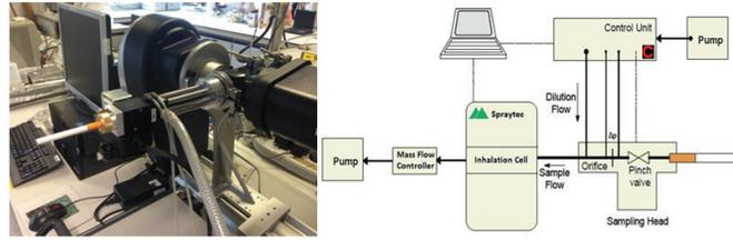
Figure 1 : Combustion Smoking Cycle Simulator / Malvern Spraytec laser diffraction (LD)
