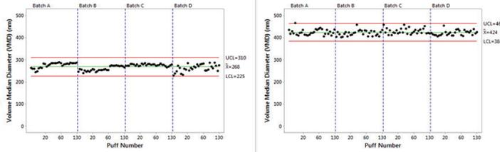
Figure 3 : Droplet diameter precision for e-cigarette @ 1:8 dilution (Intellicig, CN Creative, UK) : Electrical Mobility (left) versus Laser Diffraction (right)
